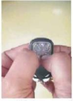
4.Resume: When remove the code carelessly, press Starting and Searching at the same time, LED starts flashing steadily after 5 seconds, release both buttons and the code will be resumed successfully.
